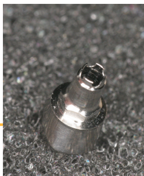
Figure 6: Implant abutment inner “fingers” at the implant connection zone.
